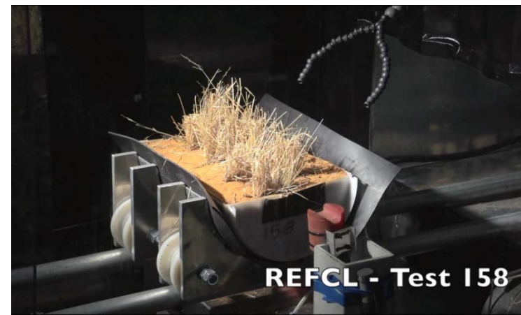
REFCL Ground Fault
