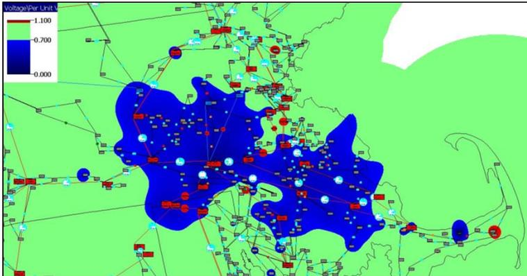
Voltage profile for 345 kV fault in East Mass., all BPS power plants **online**
