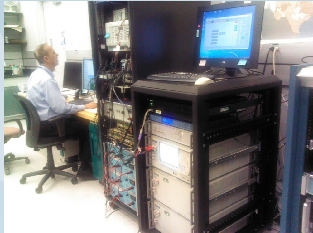
Far left: Jerry Stenbakken, middle: NIST's first PMU dynamic test system, far right: commercially available, fully automated PMU calibration system.
