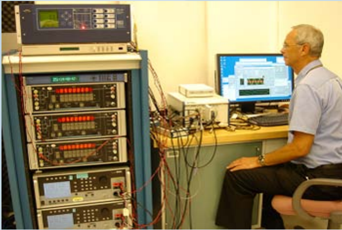
Jerry Stenbakken and the first NIST PMU steady state calibration system
